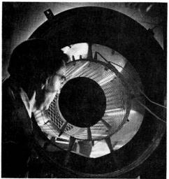
HEATER SYSTEM is shown in place inside the altitude chamber. Ken Peters checks the current control.
